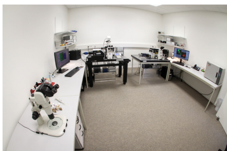
Demonstration facility with two VisiScope confocal based on Zeiss Observer and Nikon Ti microscope
