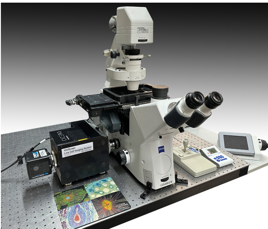
VisiScope Confocal based on Zeiss AxioObserver, CICERO confocal and Prime BSI-Express
