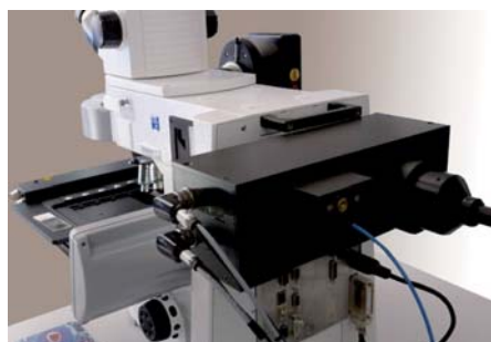
VisiFRAP mounted on Zeiss Axio-Imager upright microscope
