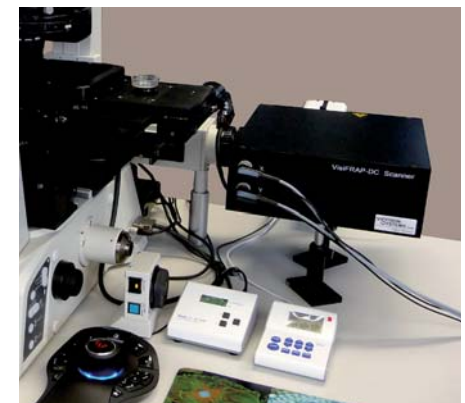
Nikon-Ti microscope with VisiFRAP-DC 355nm
