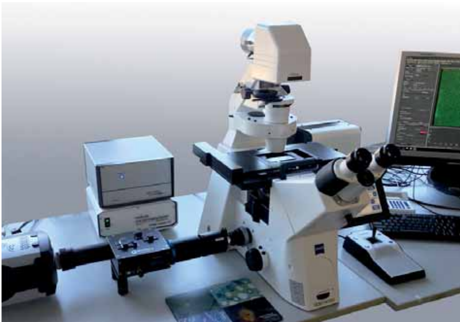
Zeiss Axio Observer with Cairn Optosplit Imager for realtime FRET analysis
