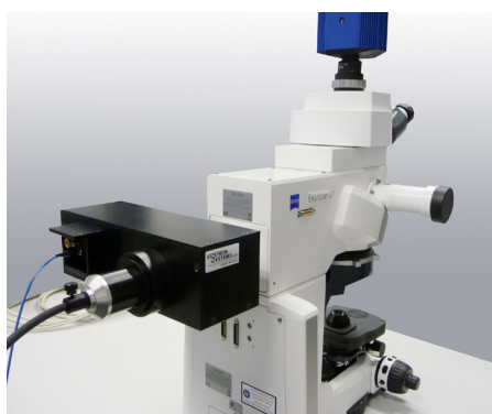
Zeiss Axi-Examiner upright microscope with VisiFRAP-2D scanner
