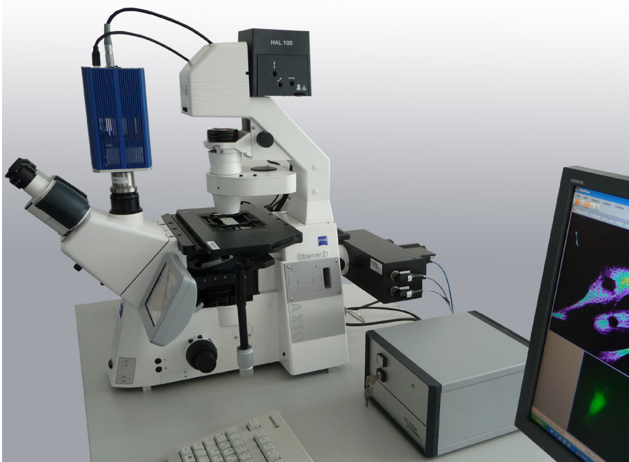
Zeiss Axio-Observer microscope with VisiFRAP-2D Scanner
