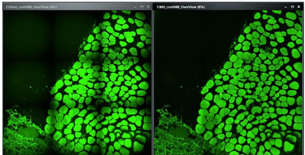
Figure 2: Scan slide acquisition of 3x3 GFP images with 13x13mm field of a sCMOS camera before shading correction and after correction
