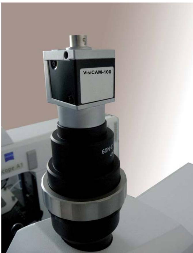
VisiCAM-100 mounted on Zeiss microscope
