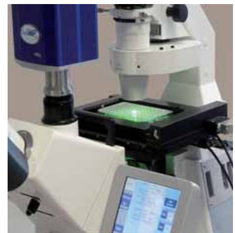
Axio-Observer with motorized XYZ-stage for multiwell scanning.
