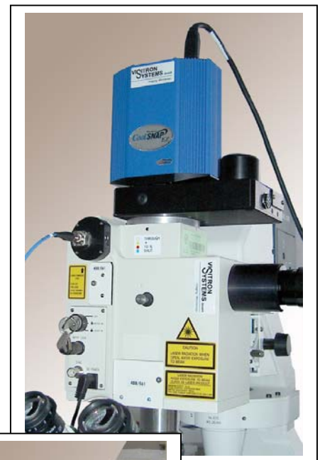
CSU10 confocal with emission-filterwheel
