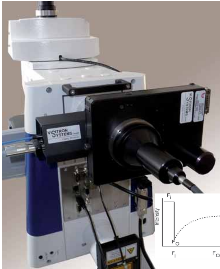
Zeiss Axio-Imager with 1D FRAP optics and motorized emission filter wheel.
