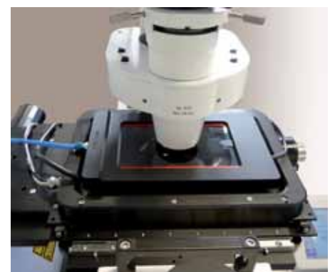
Small incubation system with heating universal Labtek holder and heating CO 2 -cover.
