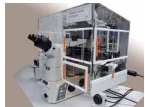
Nikon Ti microscope with PFS perfect focus and large XL incubation chamber, CSU-X1 with sCMOS PCO Edge.
