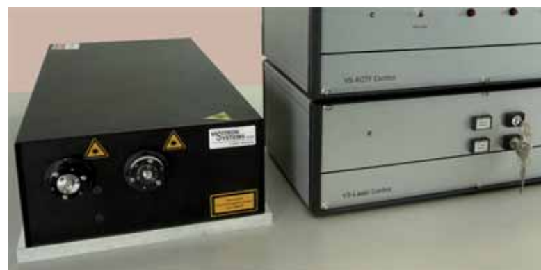
VS-LMS3 laser merge system with a Galvo dual laser output for confocal and FRAP.
