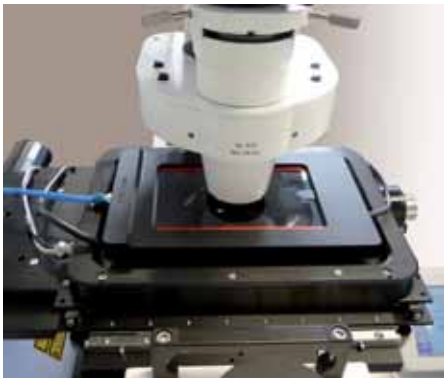
Small incubation system with heating universal Labtek holder and heating CO 2 -cover.
