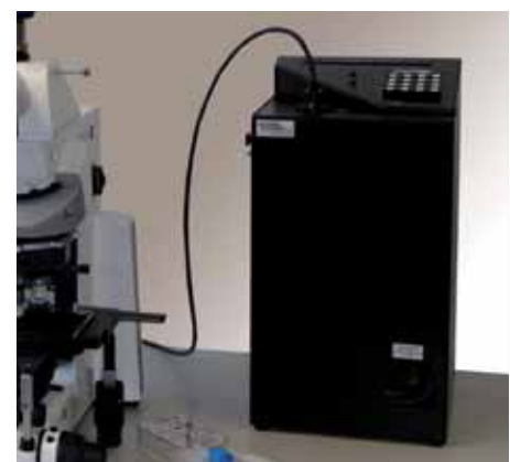
DG-4 high speed illumination system with 300W power.
