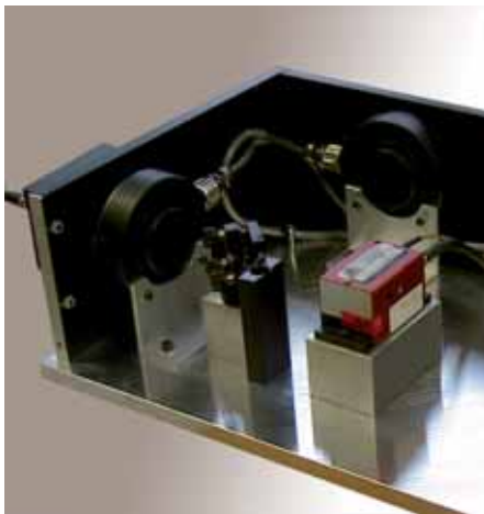
AOTF with dual laser output and high speed laser shutter.
