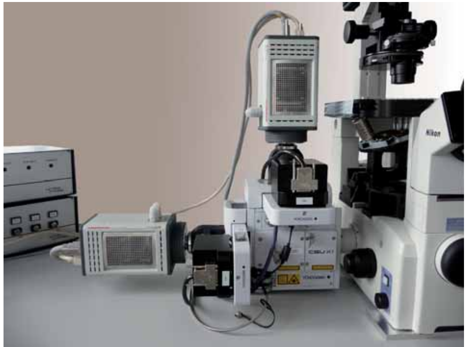
Nikon TE with CSU-X1 and dualcam option with ORCA-EM camera and VS-LMS.
