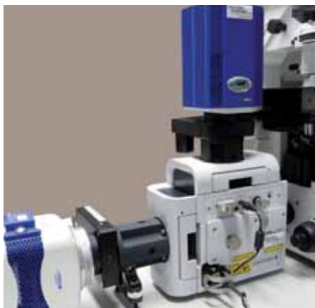
CSU-X1 confocal with VS filter wheel.
